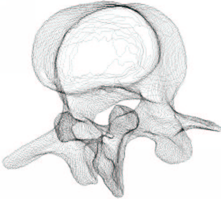
Figure 5: A Radial Basis Function is fit to this set of surface points to create a virtual vertebrae surface. The RBF automatically interpolates through the areas with low point density.
