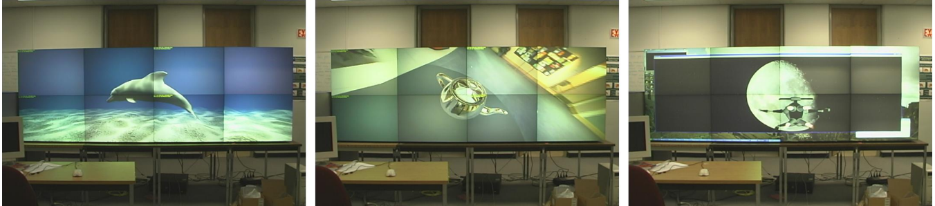
Figure 1: Unmodified Direct3D samples running on an 8 projector wall. Fullscreen and windowed modes and cubemap support is shown.
